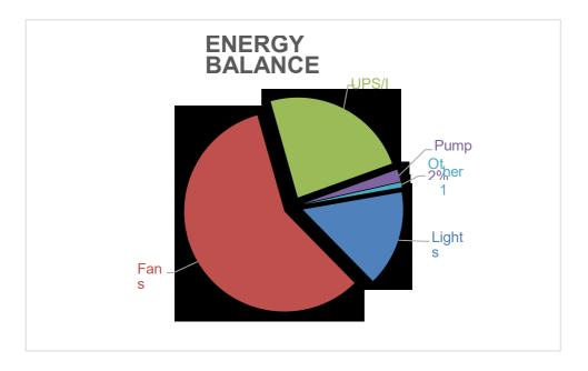
58 % of the total energy consumed in this facility is used to operate Fans. Lighting uses 15% Pumps uses 15%. IT Equipment uses 24% and Others uses 1%
